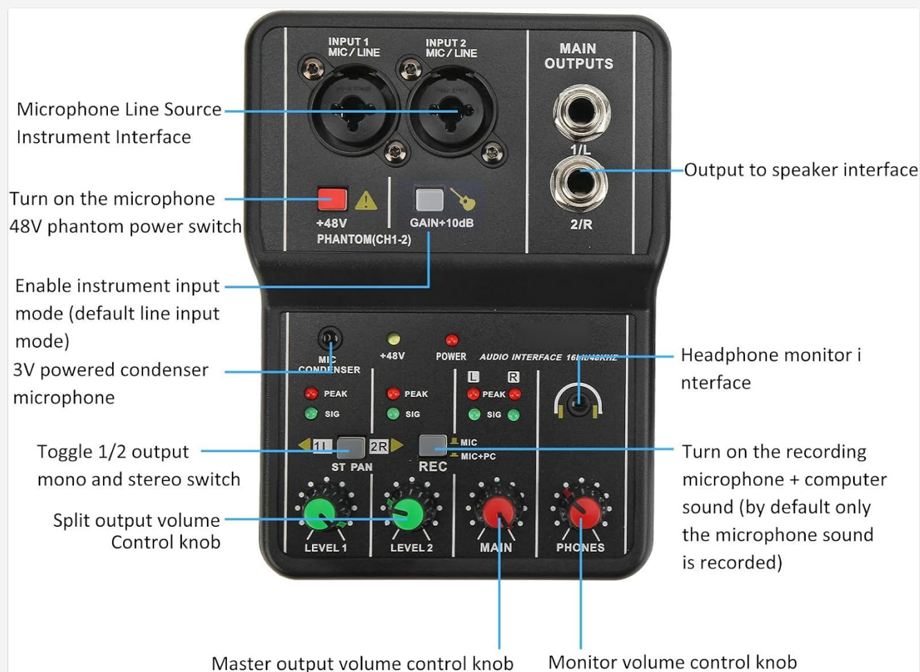
Image 4.1: Labeled diagram of the ASHATA 2 Channel Audio Mixer controls.
