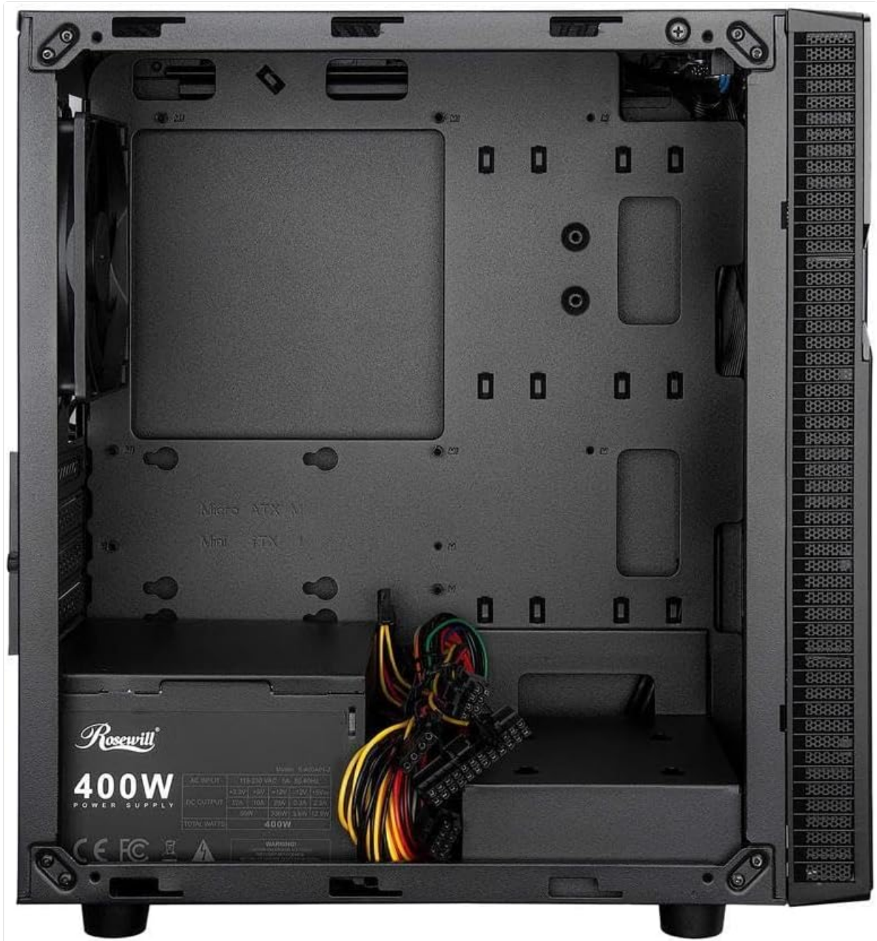
Figure 2: Internal layout of the PC case, highlighting the pre-installed power supply and available drive bays.
