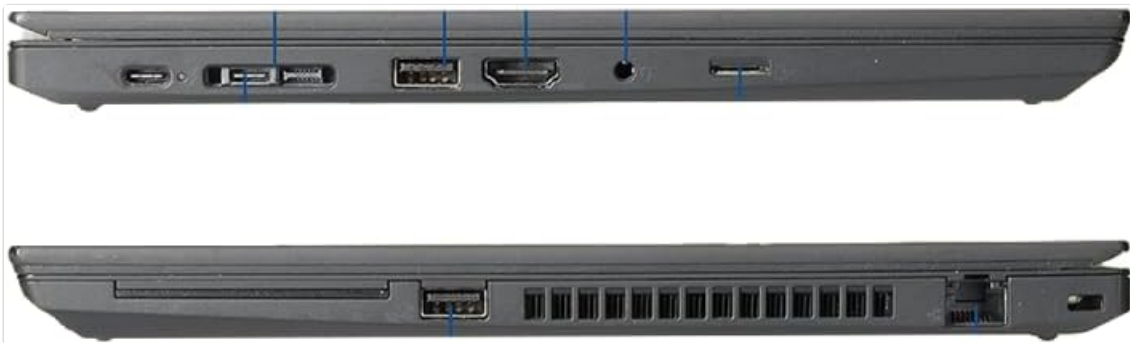
Figure 2.3: Side view of the Lenovo ThinkPad T490, illustrating the arrangement of its ports. These include USB-C (Thunderbolt 3), standard USB-A ports, an HDMI port, and an Ethernet port, among others.
