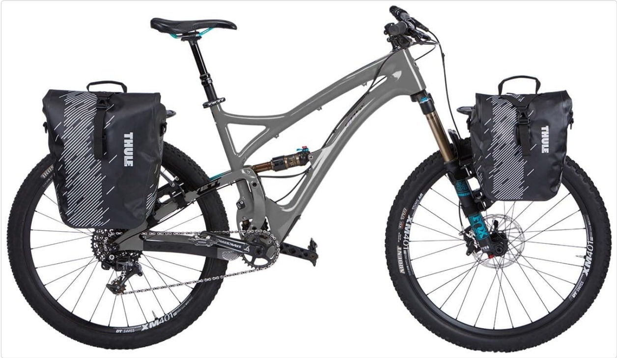
Figure 4.2: Example of the rack system with panniers, showing both front and rear installation possibilities.
