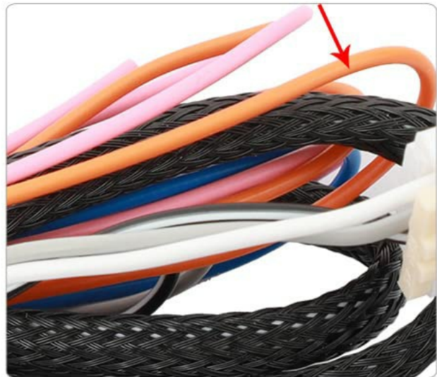
Clutch wire (optional, only connect for manual transmission cars)
