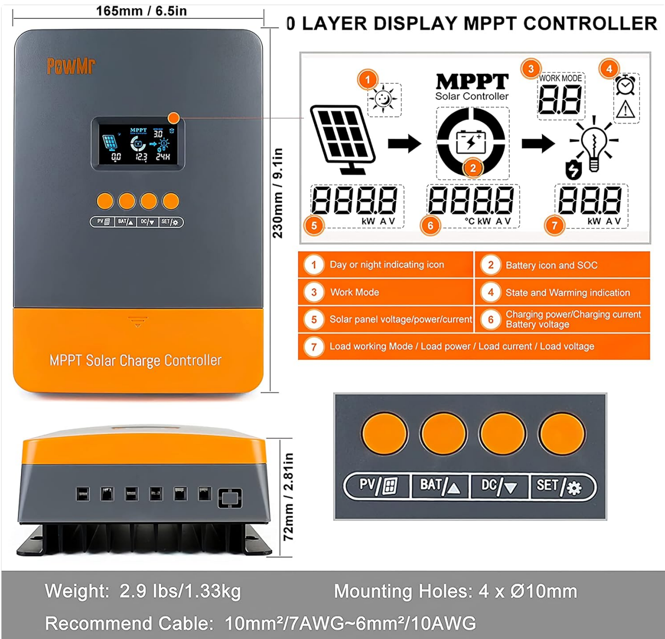
Image: PowMr MPPT 60A Solar Charge Controller dimensions (165mm x 230mm x 72mm) and its LCD display interface. The display shows solar panel voltage/power, charging current, battery voltage, and load information. Key buttons for PV, Battery, DC Load, and Settings are also visible.
