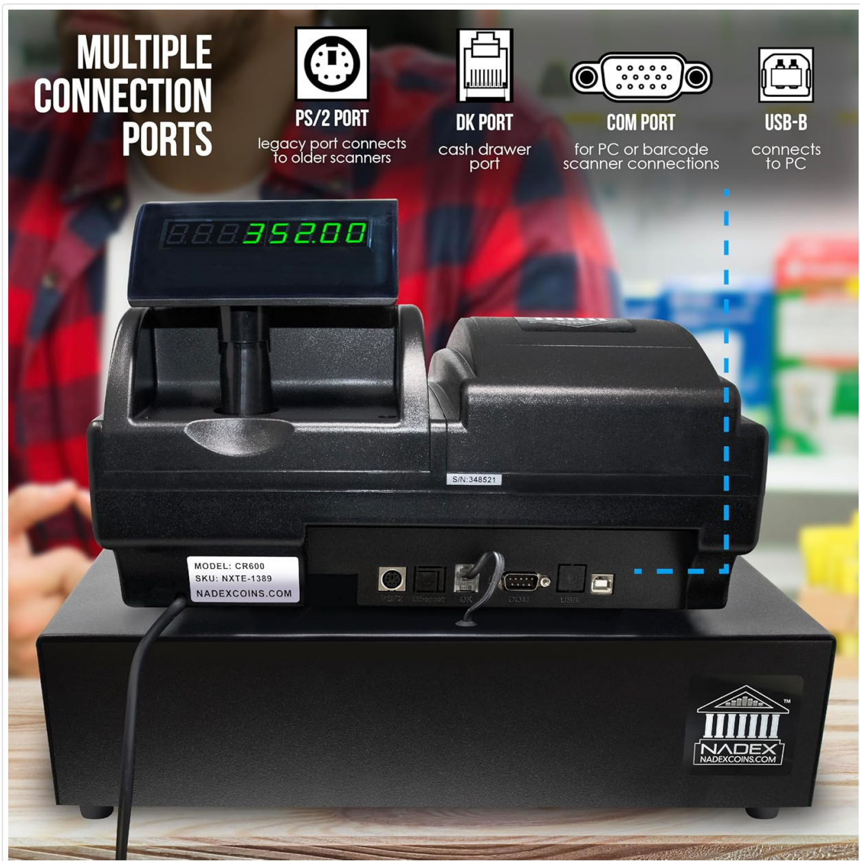
Figure 4: Rear view of the Nadex CR600 highlighting its multiple connection ports.
