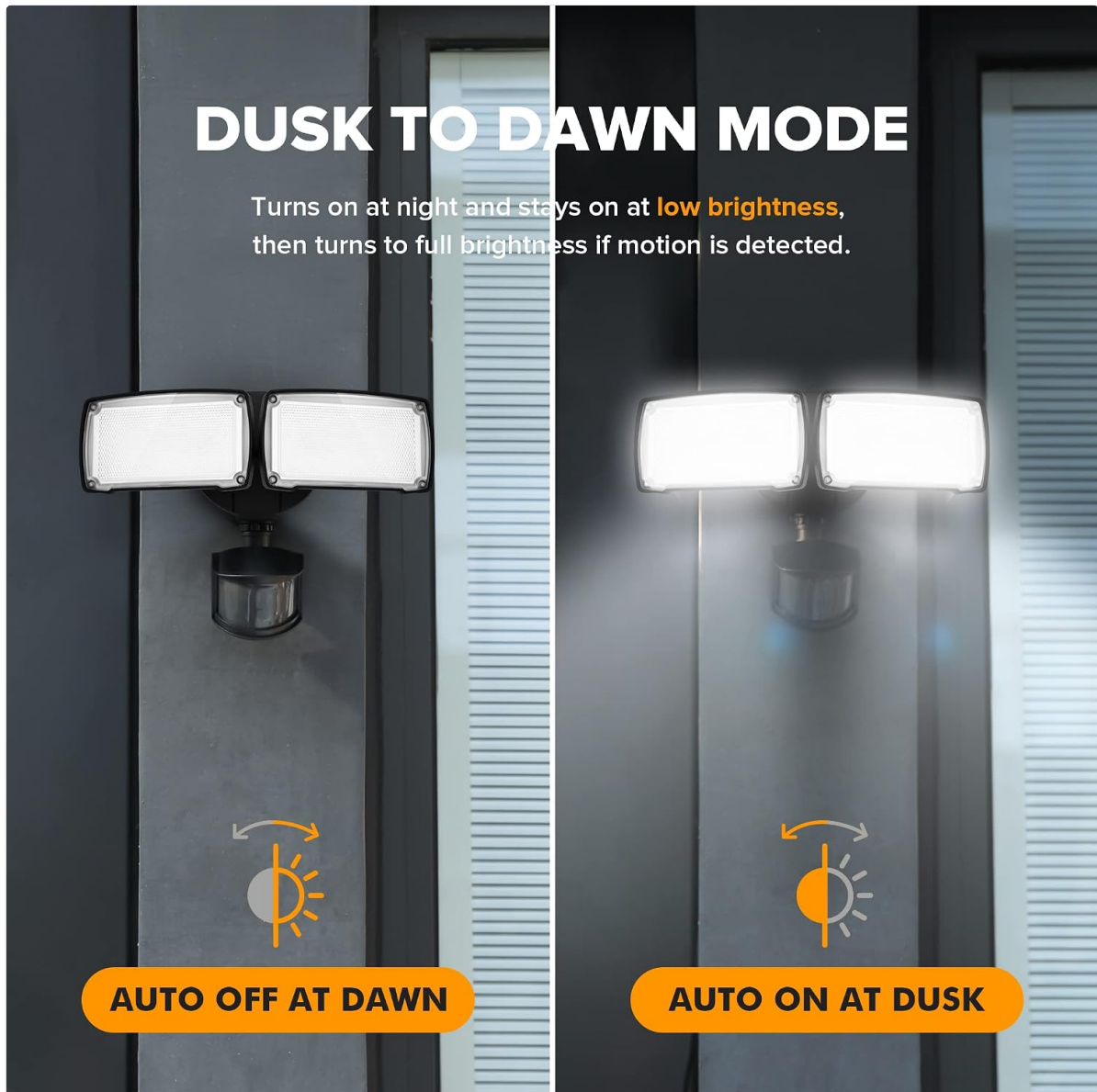
Figure 5: Dusk to Dawn Mode Operation
