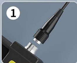
Figure 3.2: Steps for attaching the camera probe to the main unit.
