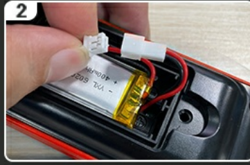
Image 3.1: Steps for connecting the internal battery before first use.
