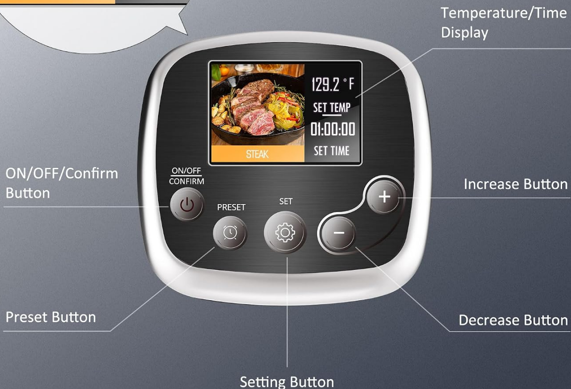
Figure 3.3: Close-up of the KitchenBoss Sous Vide Cooker's control panel, detailing the Color TFT display, temperature/time display, and buttons for ON/OFF, Preset, Setting, Increase, and Decrease. This image provides a clear view of the user interface and its various functions.
