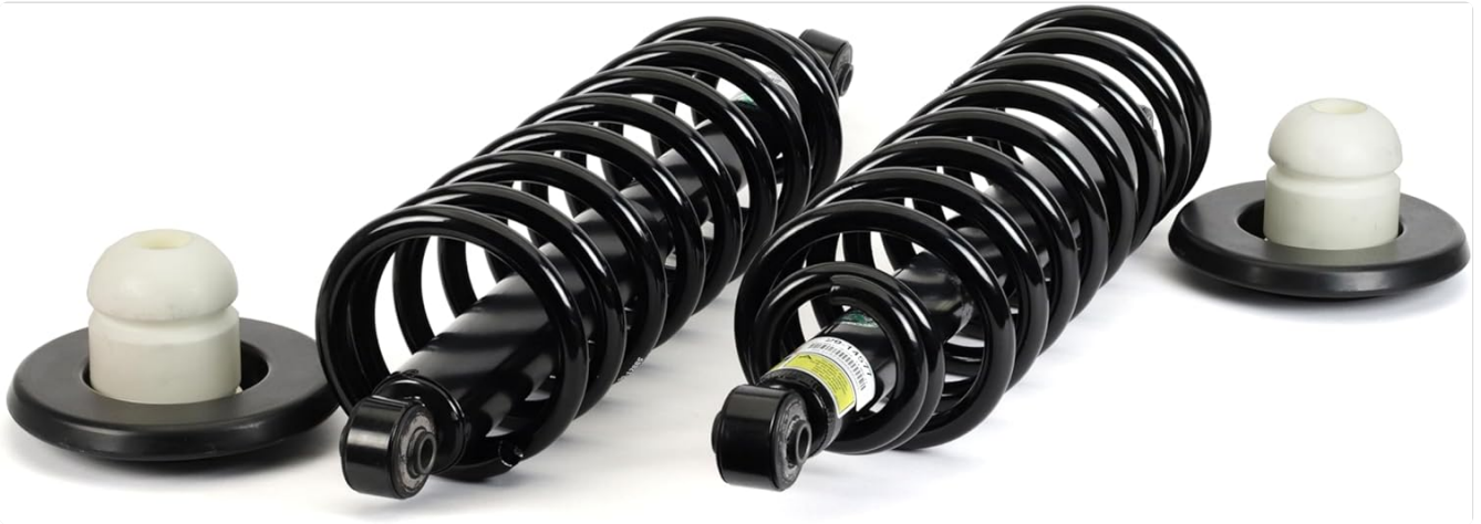
Image: Close-up of two Arnott coil springs and associated bump stops.
