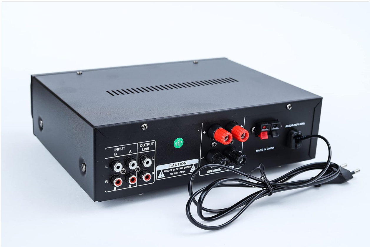
Figure 5.1: Rear panel of the amplifier, illustrating the various input (RCA), output (speaker terminals), and power connections.
