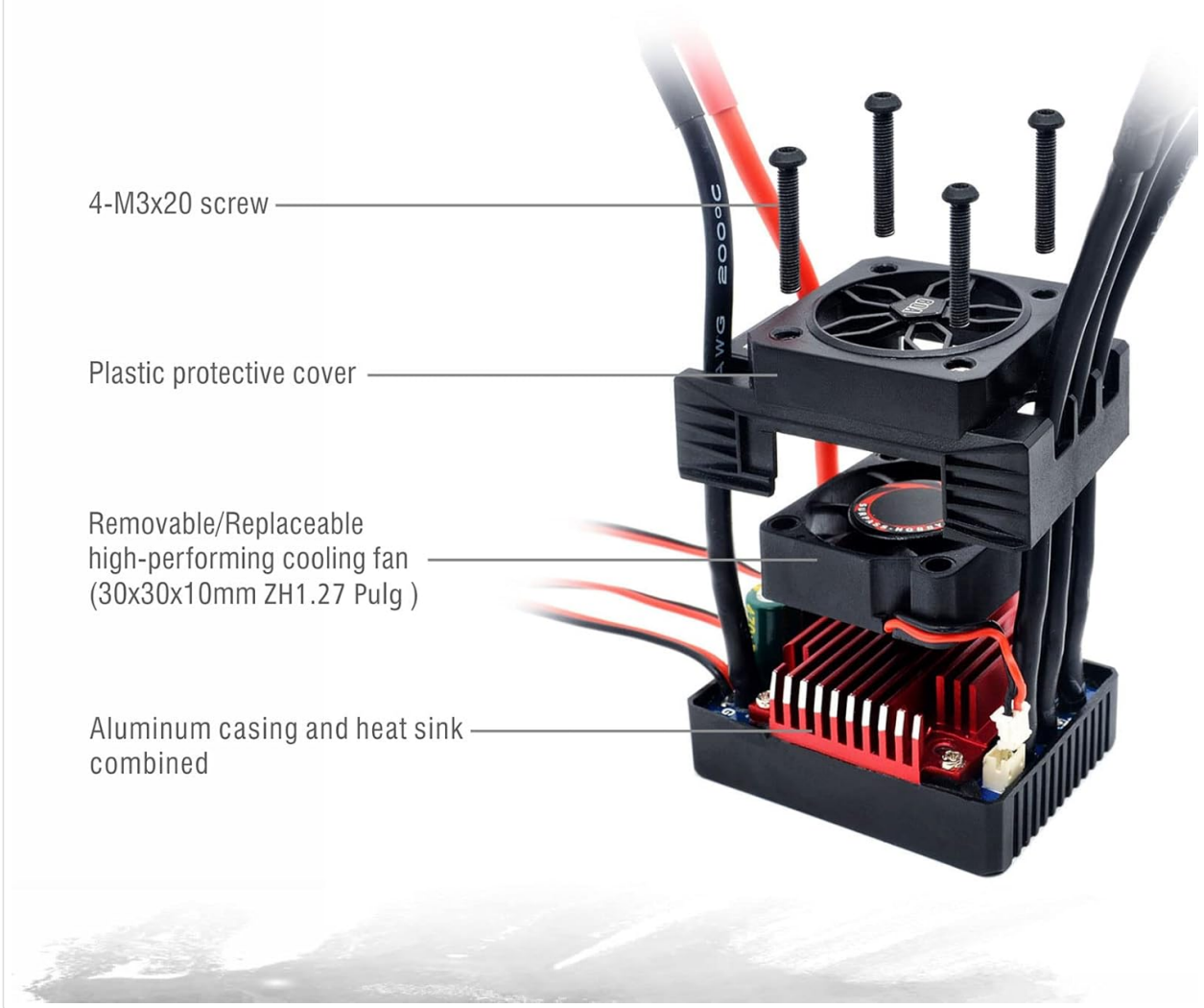
Figure 3.4: Exploded view of the ESC, illustrating its detachable design for easy cleaning and maintenance, including the plastic protective cover, removable cooling fan, and aluminum casing with heatsink.
