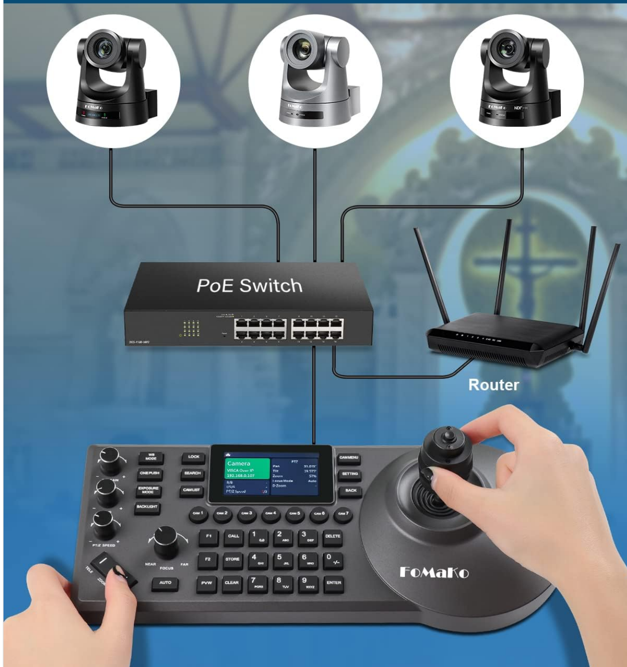
Figure 3.2: Typical System Connection Diagram
