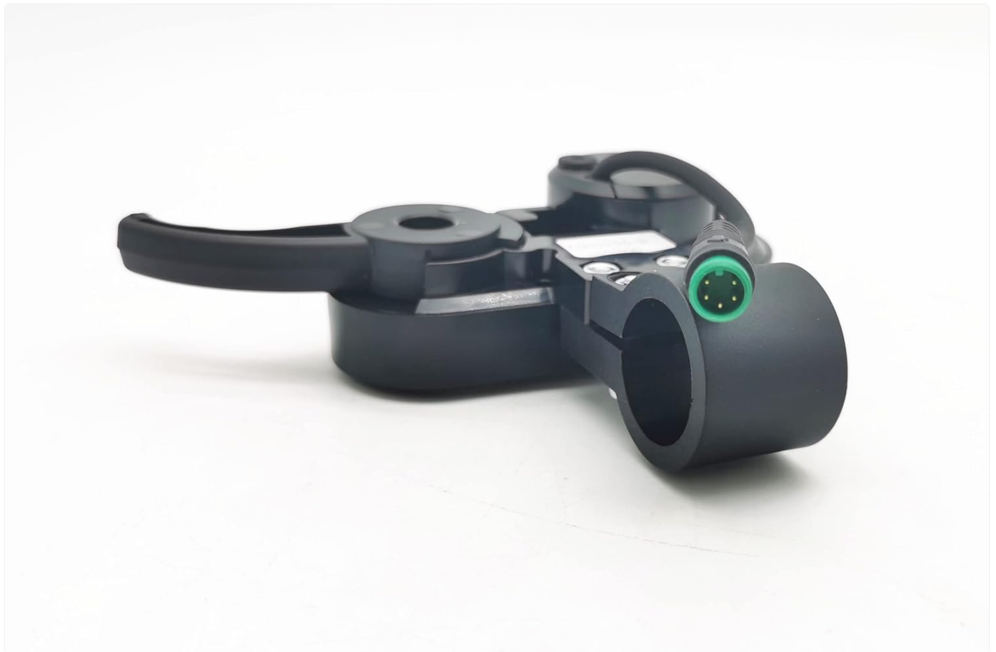
Figure 3: Side view of the TF-100 display unit, highlighting the green 5-pin connector cable.
