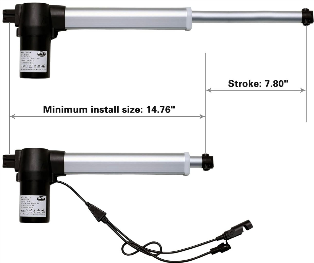
Image: Measurement guide for the RMT R811A actuator, showing minimum install size and stroke length.
