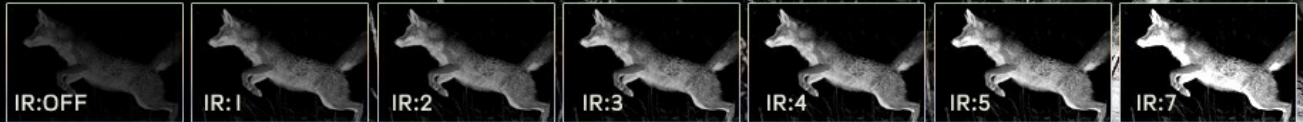
Image: Details the anti-shake and motion detection capabilities, along with the visual effect of adjusting the 7 levels of infrared illumination.
