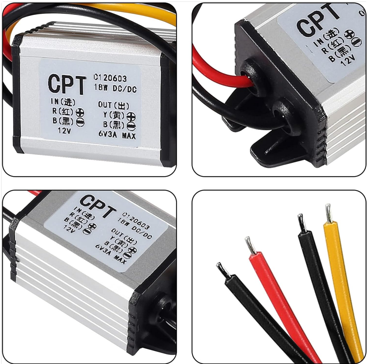
Image: Close-up view of the converter's wiring labels, indicating input (IN) and output (OUT) connections. The red wire is for input positive (+), black for input negative (-), yellow for output positive (+), and black for output negative (-).
