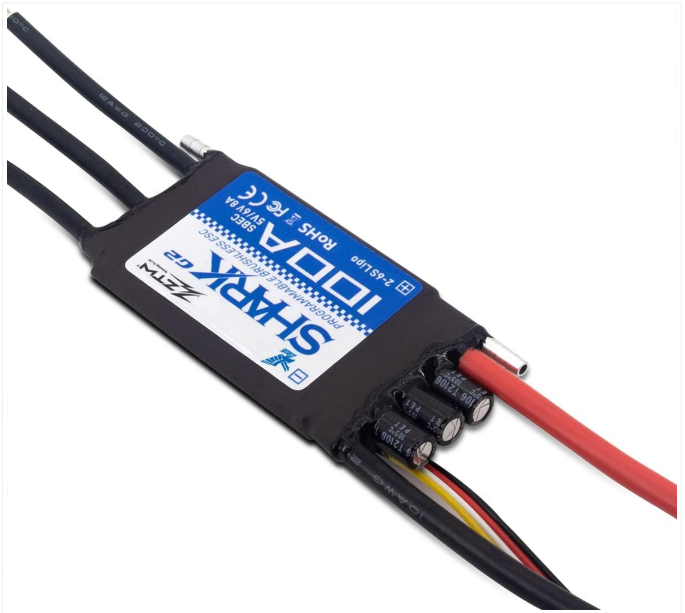
A side view of the ESC, highlighting the robust wiring for power input (red/black), motor output (three black wires), and signal (red/white/yellow), along with the capacitors.
