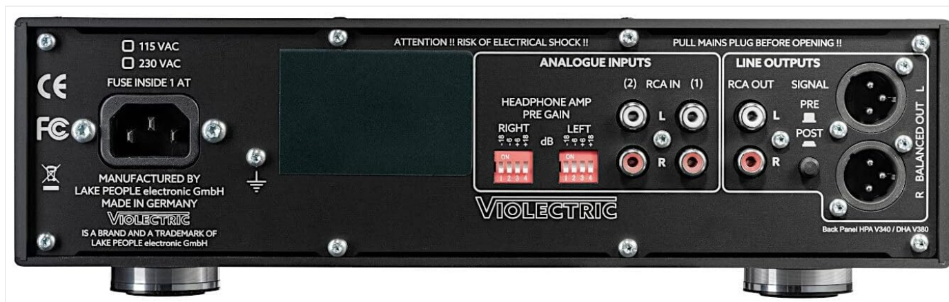
Figure 2: Rear panel of the Violectric HPA V340, highlighting the power input, 115V/230V voltage selector, RCA analog inputs, DIP switches for pre-gain adjustment, and RCA/XLR line outputs.
