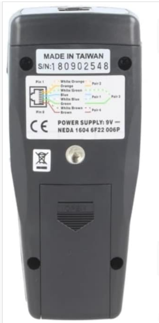
Image 4.3: Rear view of the TM-901N Main Unit with wiring diagram.
