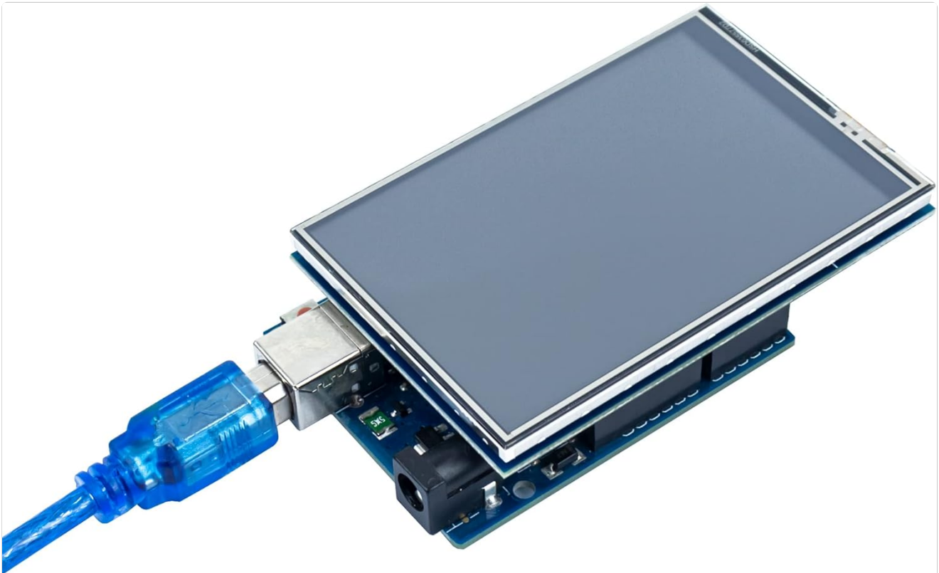
Image: The 3.5 inch TFT Touch Screen Module connected to an Arduino board, ready for operation. This demonstrates the direct plug-in capability of the shield.
