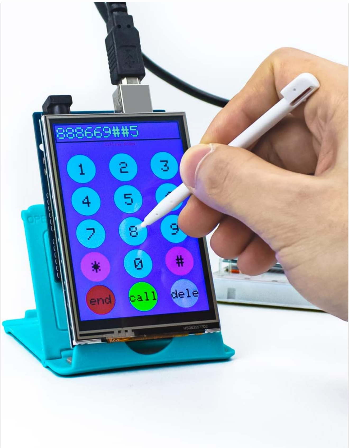
Image: A user interacting with the resistive touch screen using the provided stylus, demonstrating its input capabilities for applications like a numeric keypad.
