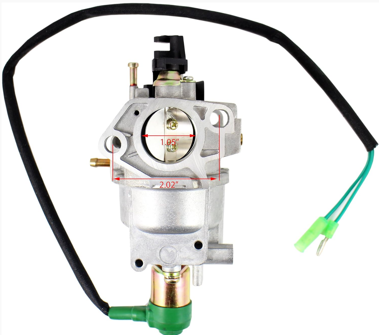
Image 2: Carburetor view with key dimensions for verification.
