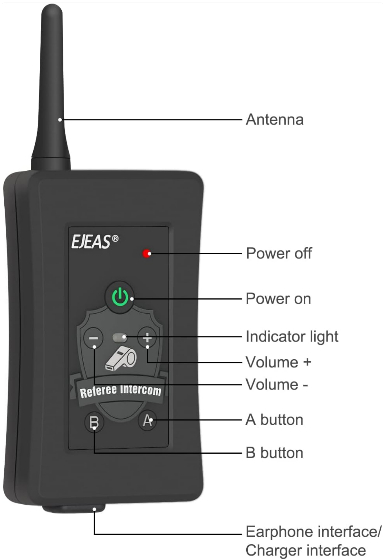
Image 3.1: Labeled diagram of the EJEAS FBIM intercom unit.
