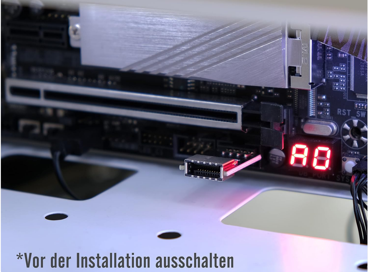
Figure 5.1: Adapter installed on motherboard
