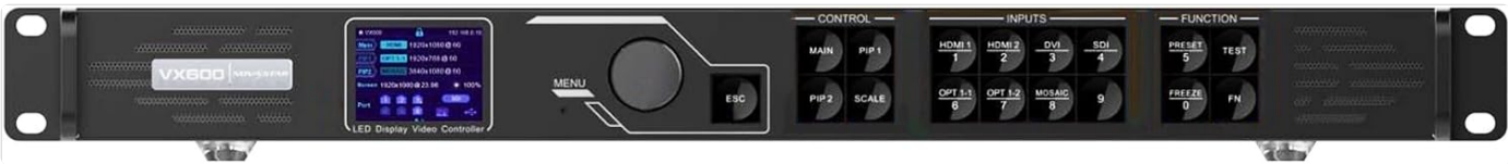
Figure 3.1: Front panel of the Novastar VX600. This view highlights the integrated display screen, the central control knob and ESC button for menu navigation, and dedicated buttons for input selection (HDMI, DVI, SDI, OPT1) and function controls (MAIN, PIP/PBP, SCALE, PRESET, TEST, FREEZE, FN).
