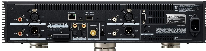
Image 3.2.1: Rear view of the TEAC UD-701N. This image details the comprehensive array of connections including XLR and RCA line inputs and outputs, Ethernet port, USB-B port for PC connection, USB-A port for USB drive, coaxial and optical digital inputs, 10MHz clock input, and the AC power inlet.
