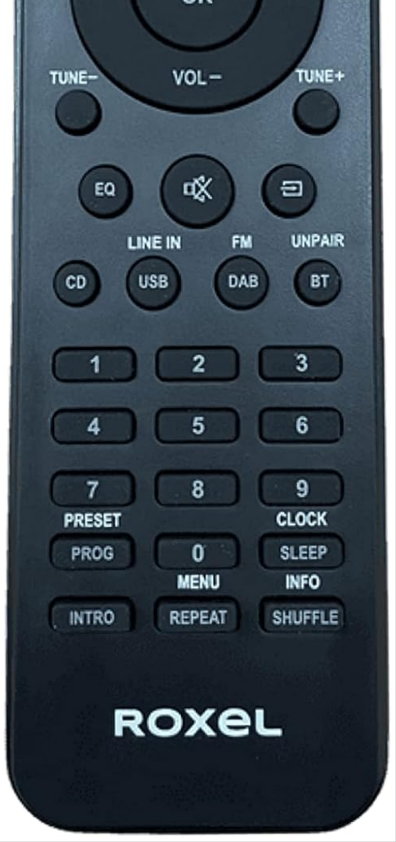
Figure 2.1: Front view of the Roxel RC-3 Universal Remote Control. This image displays the front of the Roxel RC-3 Universal Remote Control, featuring its ergonomic black design and clearly labeled buttons for various functions such as power, volume, track control, source selection, and numerical input.
