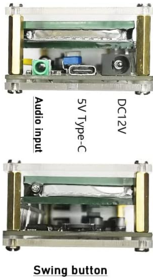
Figure 1: Top-down view illustrating the power and audio input connections.
