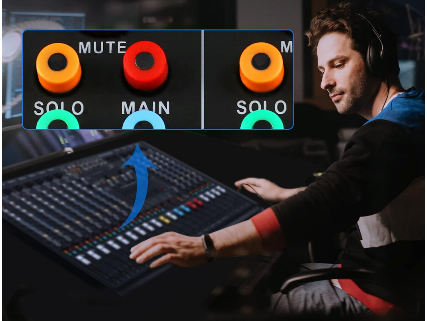
Figure 3: Close-up of the independent SOLO key. Pressing this button allows monitoring of a specific channel through headphones without affecting the main mix, crucial for sound checks and precise adjustments.
