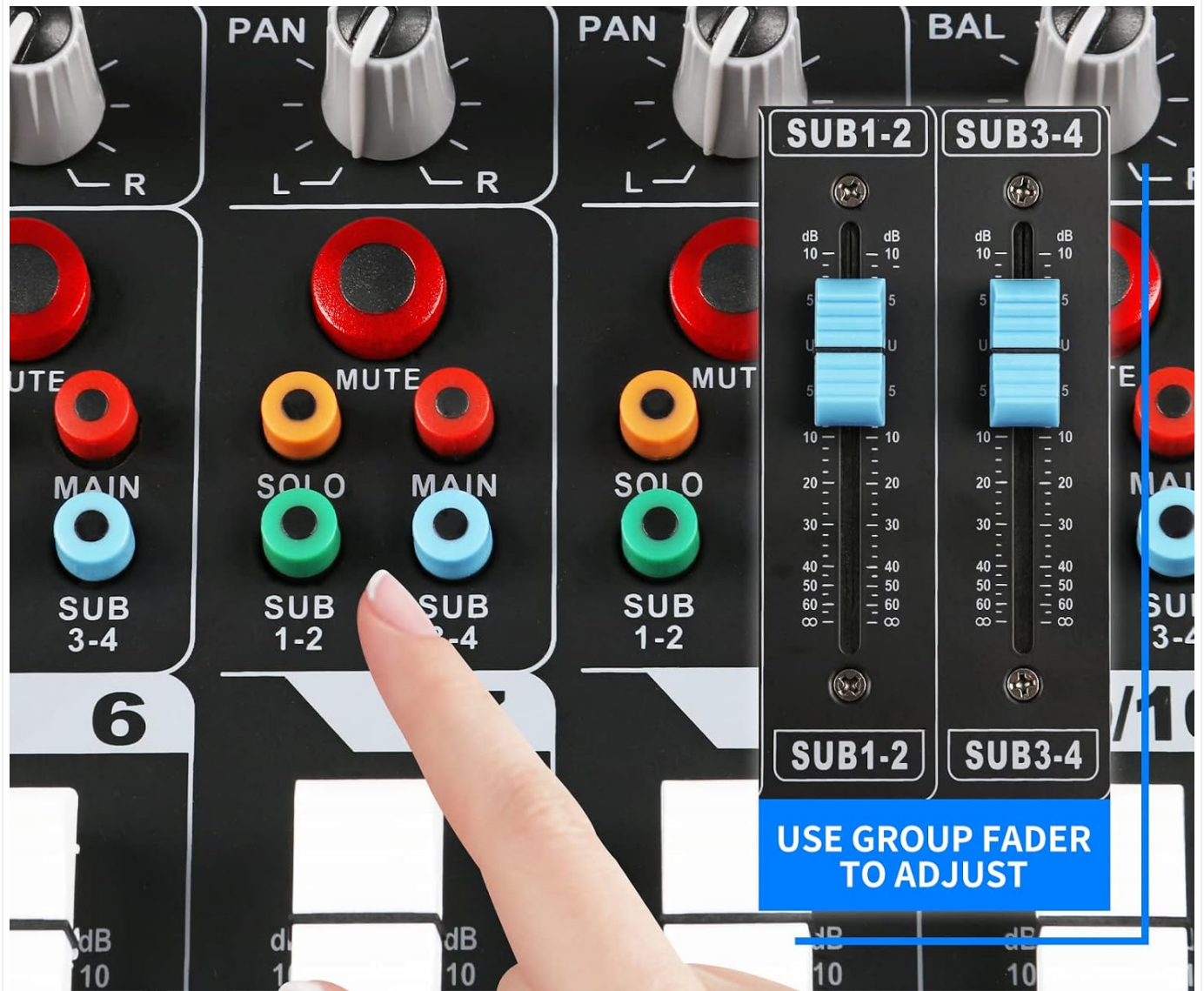
Figure 5: Detail of the 4 group output controls. These controls enable signals from multiple channels to be mixed into a sub-group, offering flexible routing and control over specific instrument or vocal sections.
