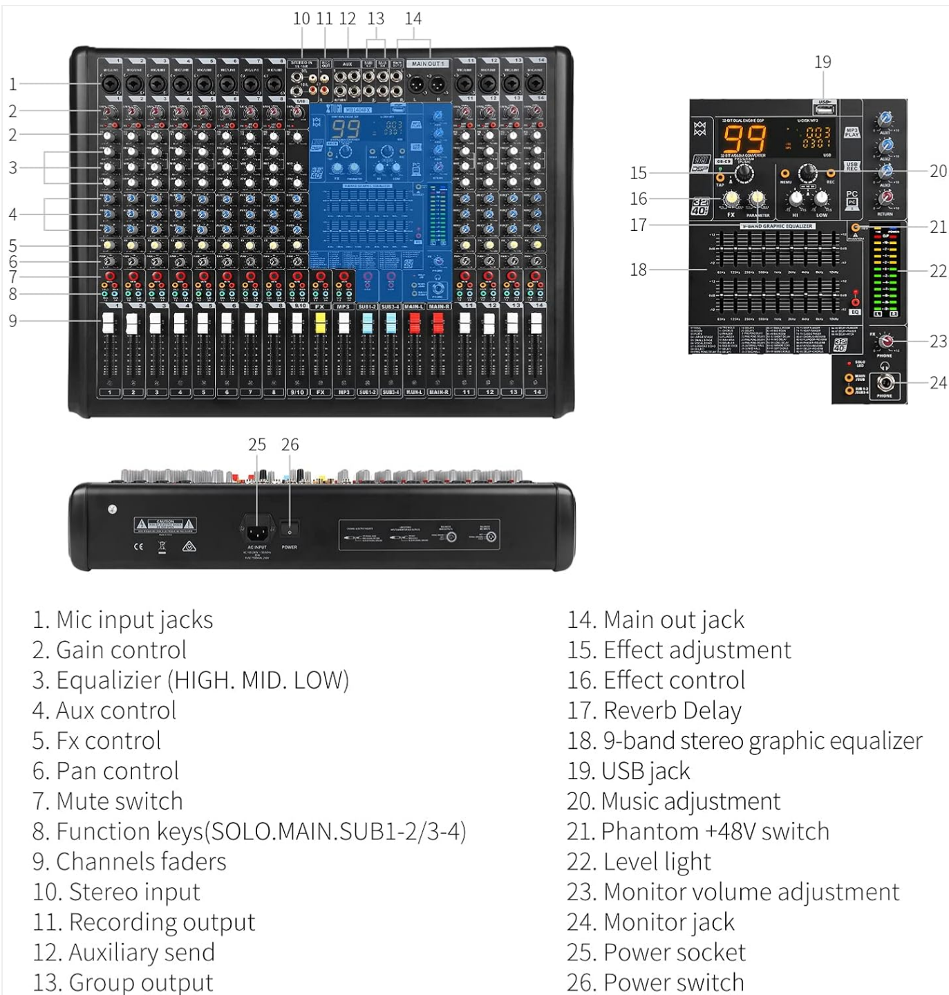
Figure 9: Detailed labeled diagram of the XTUGA MB1404FX mixer's front panel and rear connections. Each control is numbered for easy identification and reference in the operating instructions.
