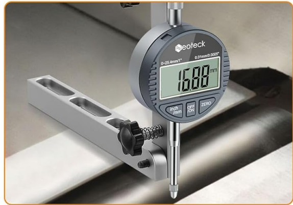
Check Jointer Depth of Cut
