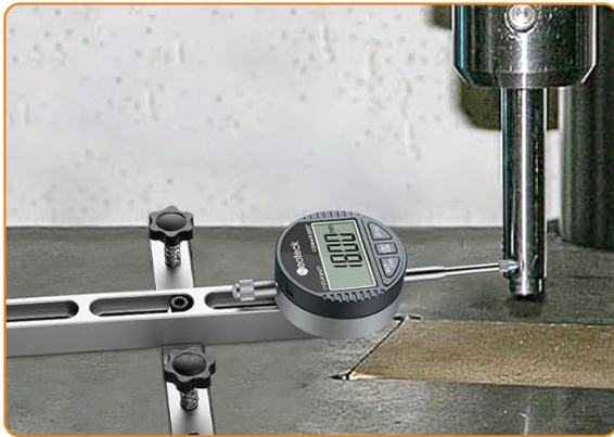
Check Drill Chuck Run-out
