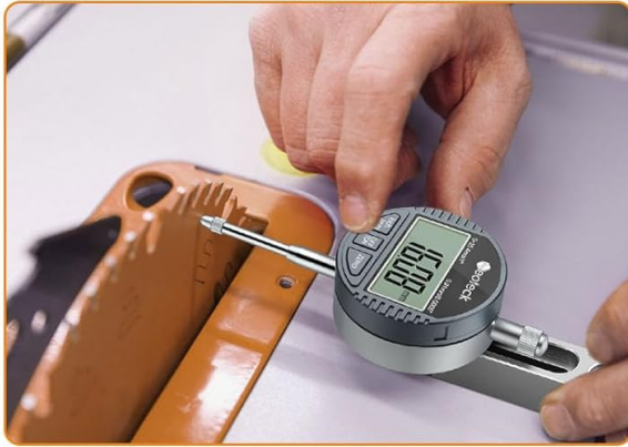
Check Saw Blade Alignment and Run-out
