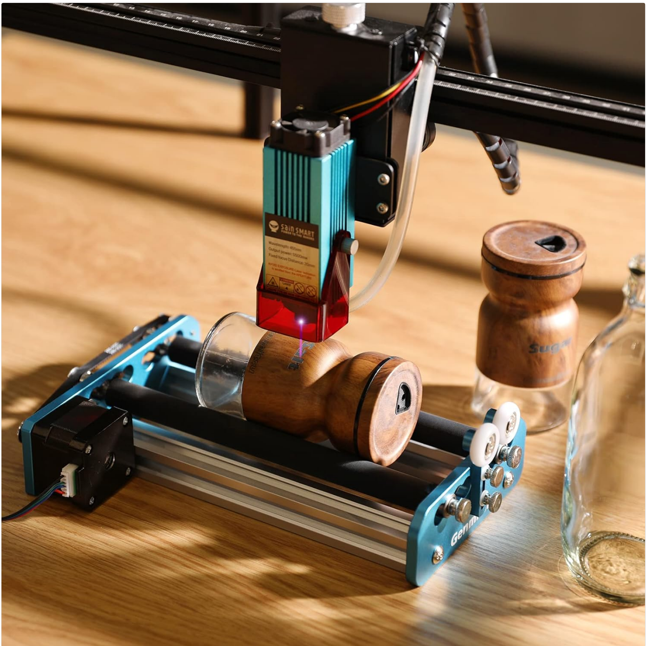
Figure 6: The Genmitsu Laser Rotary V2 in operation, precisely rotating a wine glass as a laser engraver applies a design.
