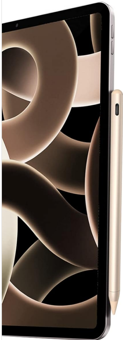
Figure 6: The stylus magnetically attaches to the iPad, allowing for convenient charging even while attached, thanks to its accessible USB-C port.
