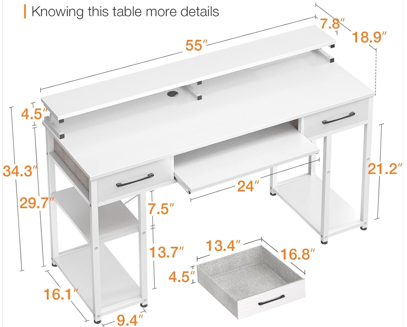
Figure 1: ODK Computer Desk Dimensions and Key Parts. This diagram illustrates the overall dimensions of the desk and highlights various components for assembly.
