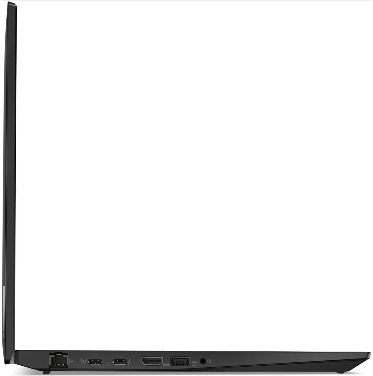
The left side ports of the ThinkPad T16 Gen 1, including Ethernet, USB-C, Thunderbolt, HDMI, and audio jack.
