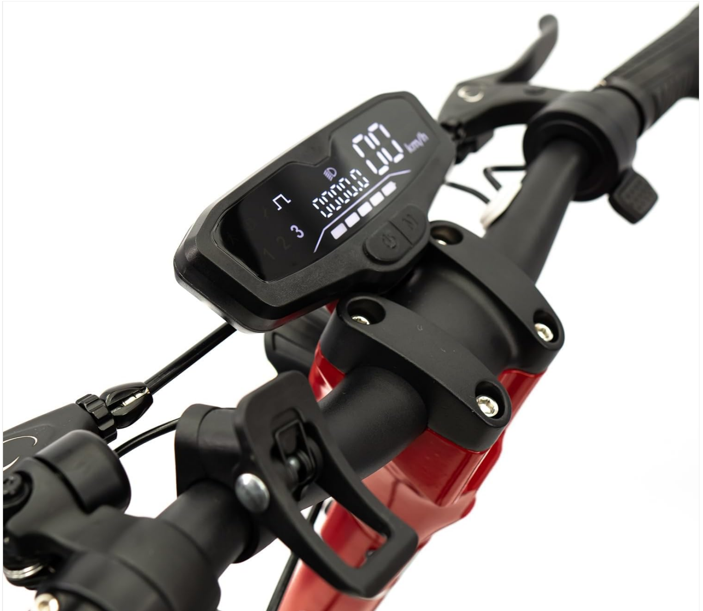
Image: Detailed view of the scooter's multifunction display on the handlebars, showing speed, battery, and odometer readings.
