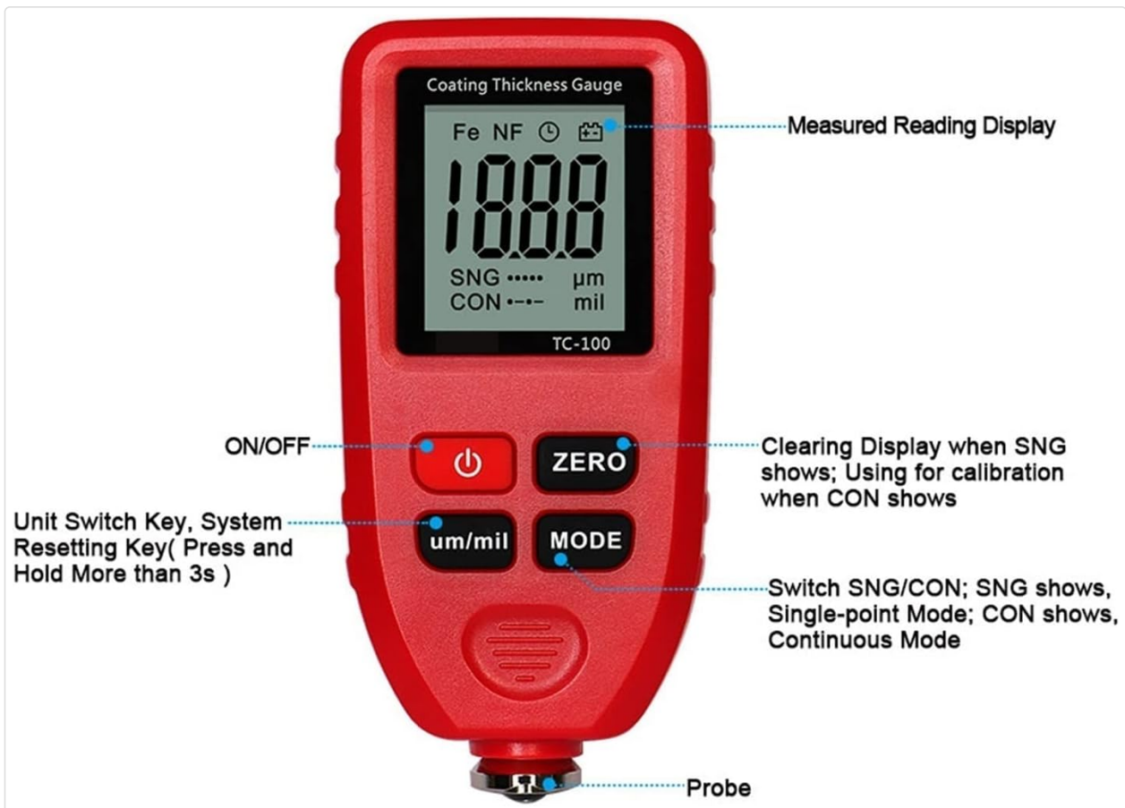
Image 4.1: Detailed diagram of the TC100 Coating Thickness Gauge, highlighting the measured reading display, ON/OFF button, ZERO button, unit switch key (um/mil), mode switch (SNG/CON), and the probe.
