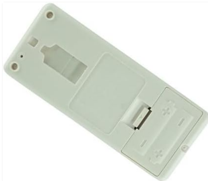
Figure 3: Back view of the remote control with the battery cover securely reattached after battery installation.
