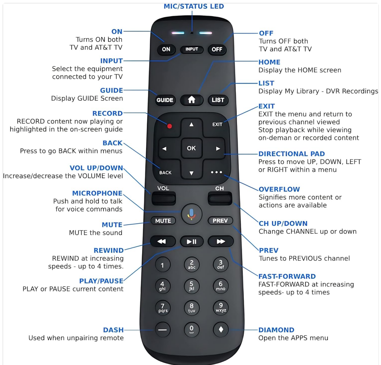
Image: Labeled diagram of the RC82V remote control buttons and their functions.
