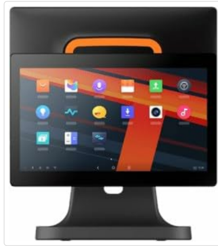
Figure 4.1: Front view of the SUNMI T2s Lite POS system. This image displays the main 15.6-inch touchscreen, which is the primary interface for operating the device. The design is compact and suitable for various retail settings.
