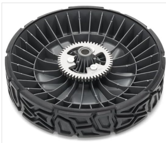
Image 2: Rear view of the Toro 140-2350 Rear Drive Wheel, showing the internal gear mechanism. This gear engages with the mower's transmission to provide self-propelled motion.
