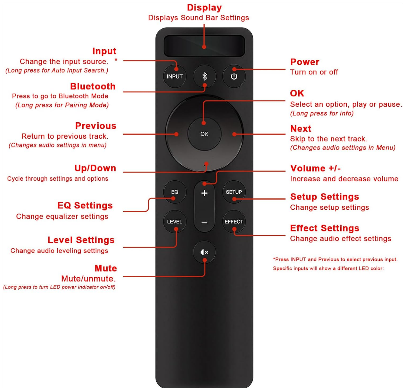
Image: A detailed diagram labeling each button on the D512-H remote control and its corresponding function.
