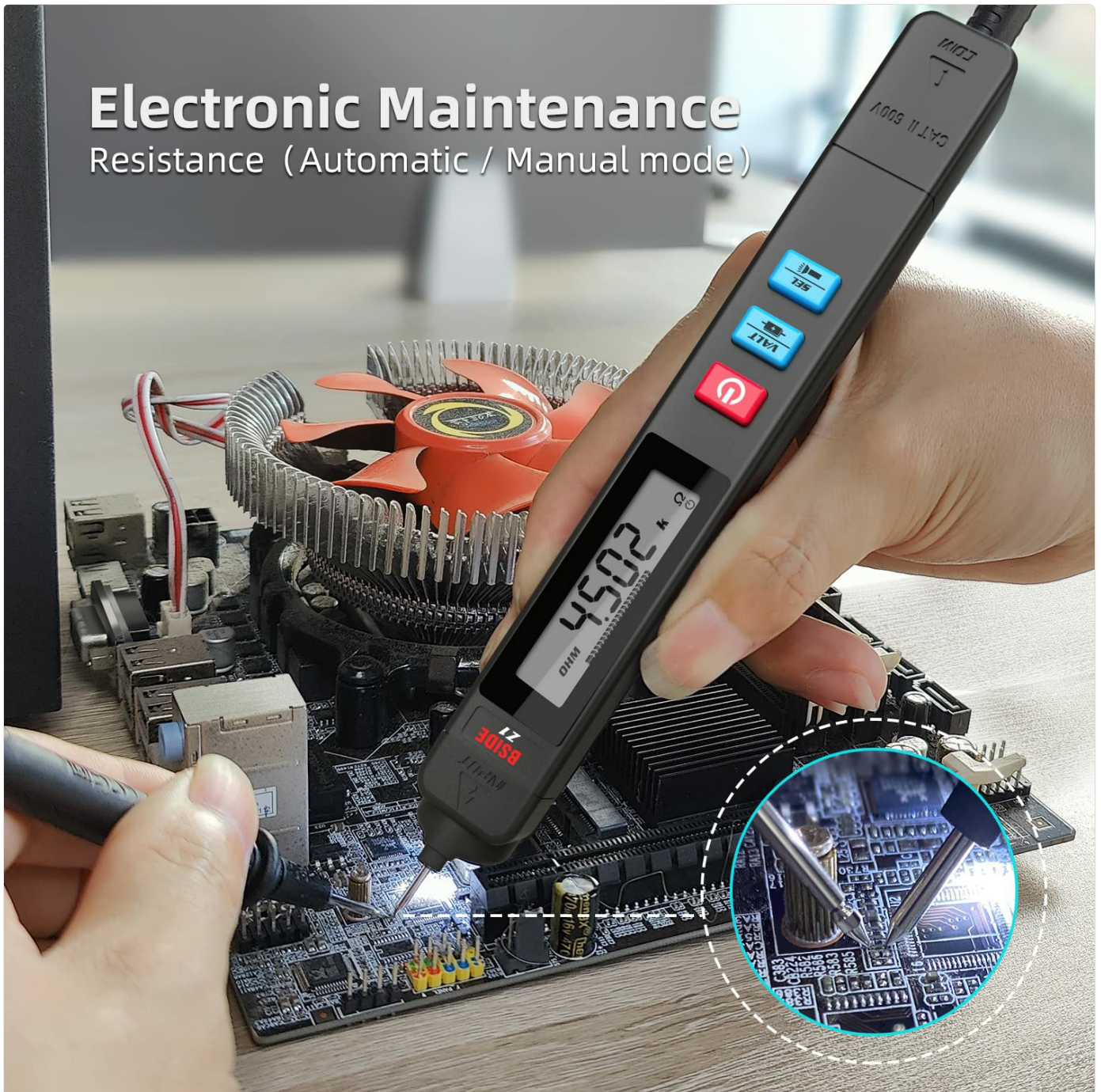
Figure 6.2: Measuring resistance on a circuit board using the BSIDE Z1 Multimeter.
