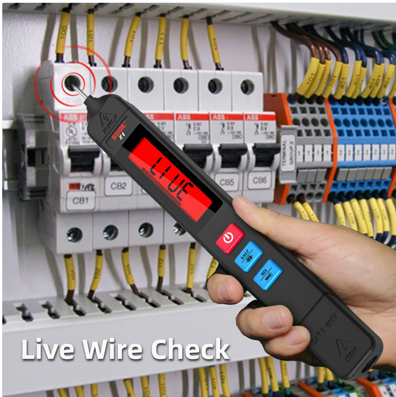
Figure 6.3: Performing a live wire check with the BSIDE Z1 Multimeter.
