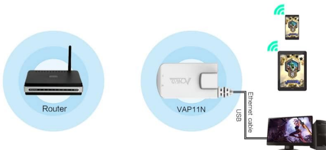
Image: Diagram illustrating the AP Mode, where the VAP11N-300 connects to a wired network and broadcasts a Wi-Fi signal for wireless devices.
