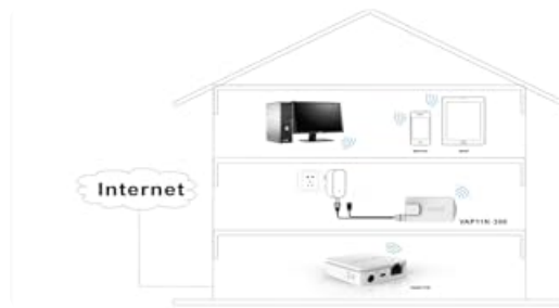
Image: Diagram illustrating the Repeater Mode, showing the VAP11N-300 extending Wi-Fi coverage within a multi-story building.
