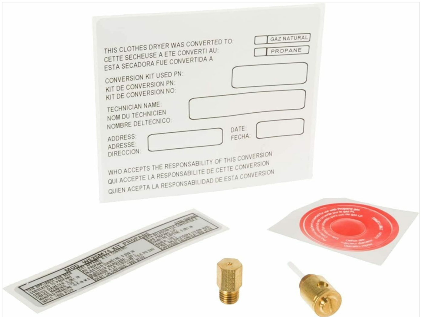
Image 3.1: Components of the WE25M74 LP Gas Conversion Kit. This image displays the LP orifice, the LP regulator component, and the conversion label, which is to be affixed to the dryer after successful conversion.
