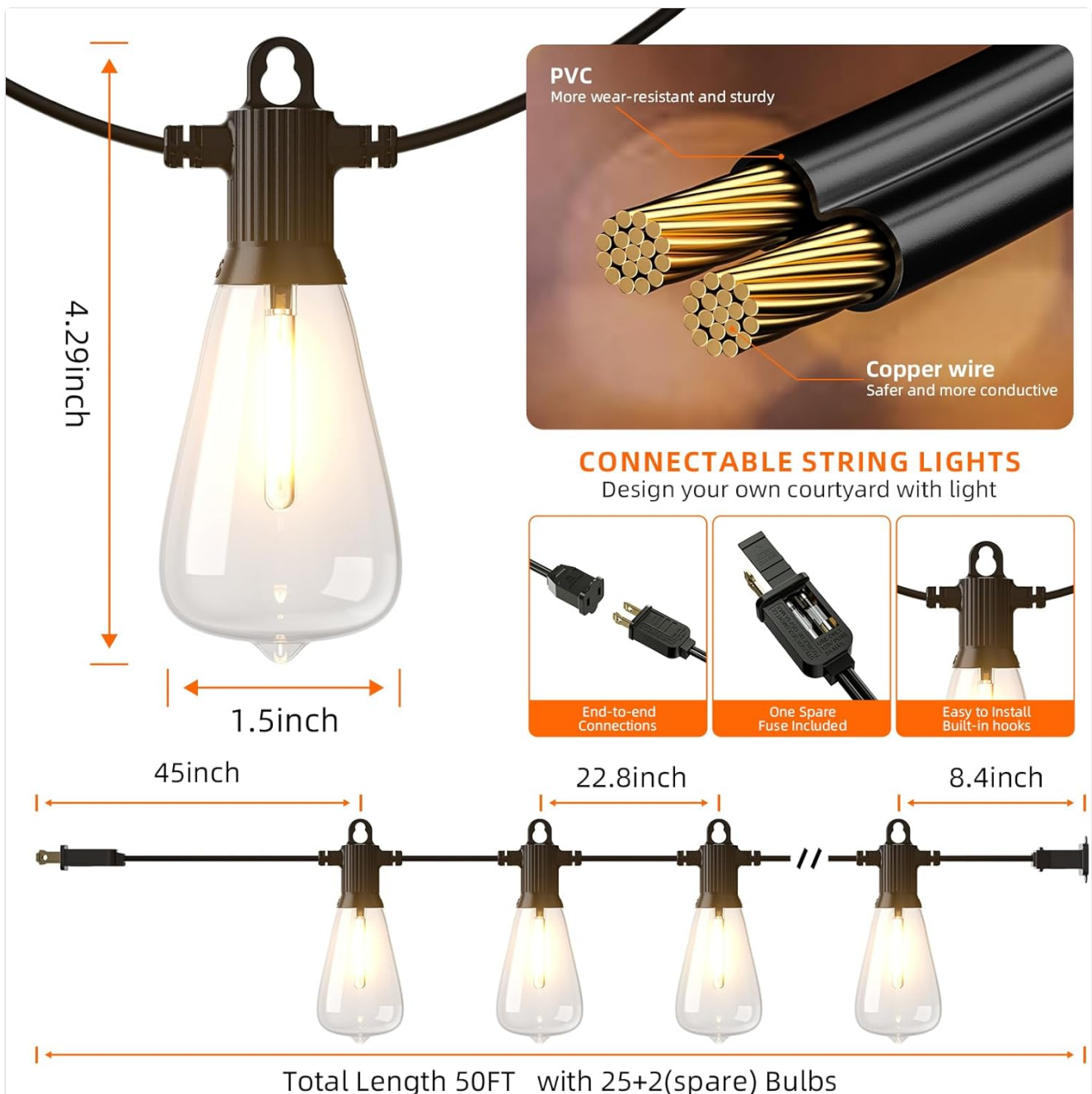
Diagram illustrating the dimensions of the 50FT string light and its end-to-end connectable feature.
