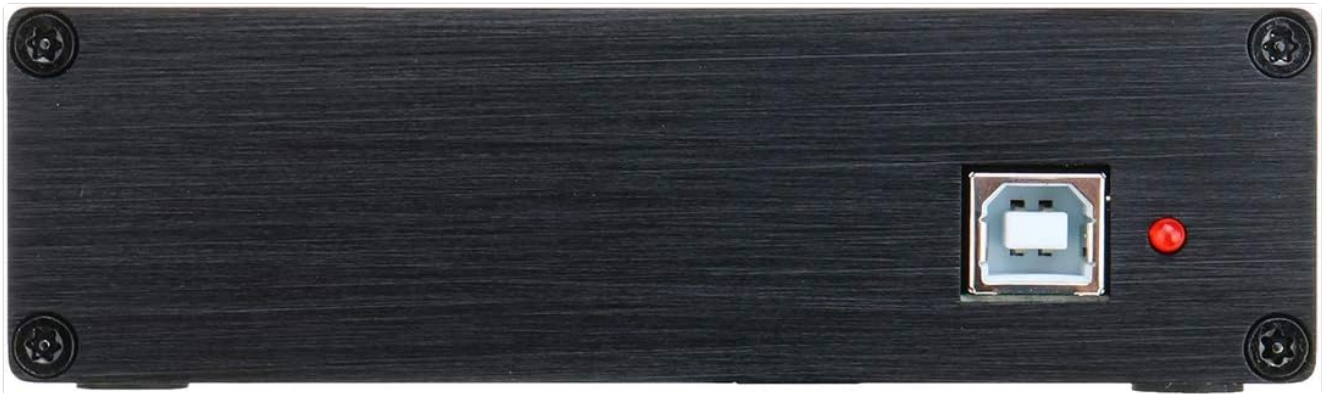
Figure 2: Rear view of the UMH-10, highlighting the USB-B "Power In" port.
