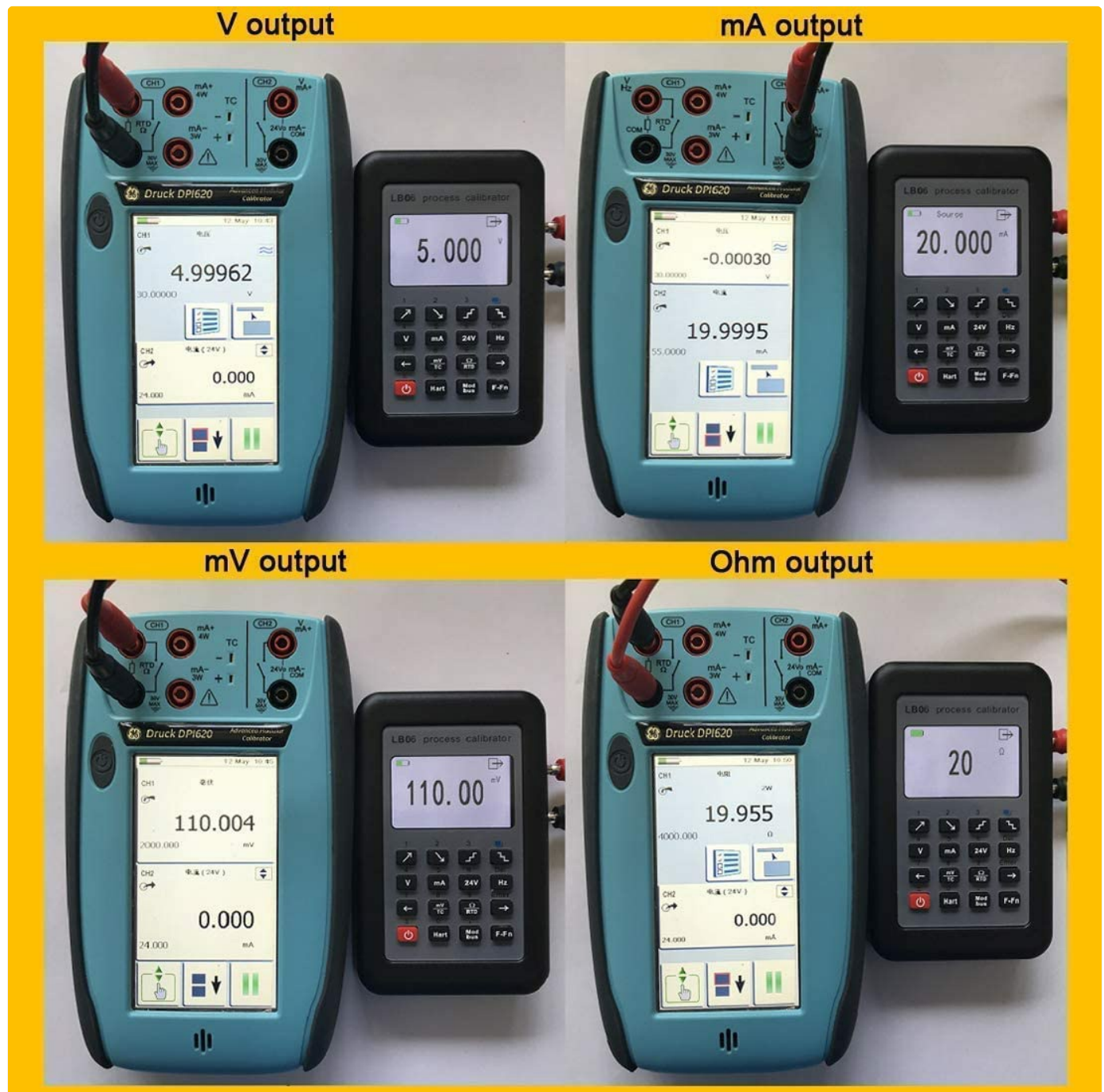
Figure 4.2: Examples of LB06 outputting Voltage (V), Current (mA), Millivoltage (mV), and Resistance (Ohm) compared to a reference device.
