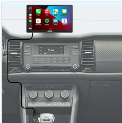
Image: Diagram showing the connection of the power cable from the P8 unit to the cigarette lighter adapter.
